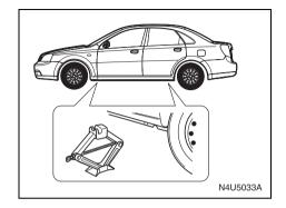
3) Near each wheel well is a notch in the frame which the jack head fits in. Position the jack and raise the jack head until it fits firmly into the notch in the vehicle's frame nearest the flat tire. Put the compact spare tire near you.
